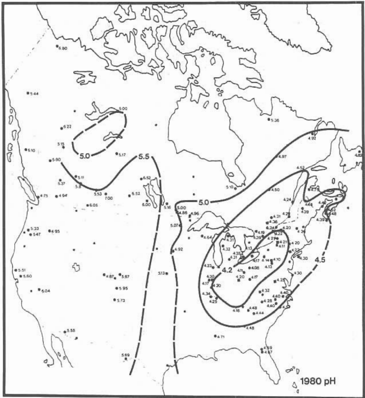
Figure 2. The spatial variation of the precipitation-amount weighted-mean pH over North America in 1980 compiled from several monitoring networks. Isopleths are dashed where the position is uncertain and omitted in regions of insufficient data. (Source: Barrie and Hales 1984).
