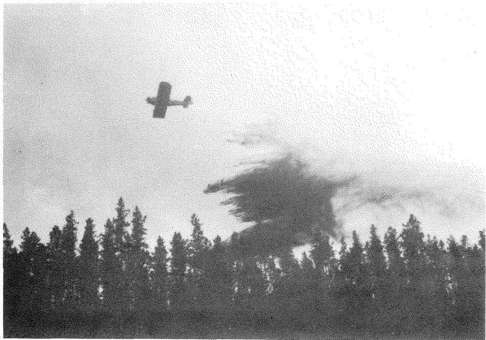
Figure 4 A high drop on the lodgepole pine stand with Fire-Trol 100.
