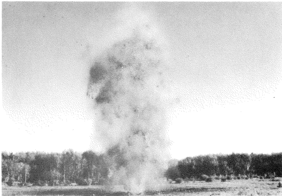
Figure 2. A Phos-Chek 205 drop on the open field grid system.
