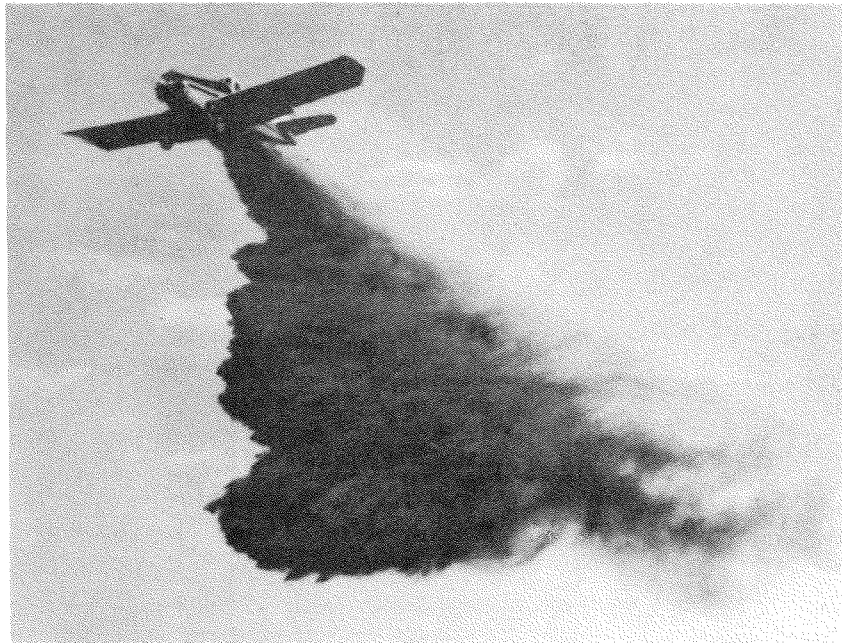
Figure 5. Thrush Commander releasing 310 Imperial gallons of thickened fire retardant.
