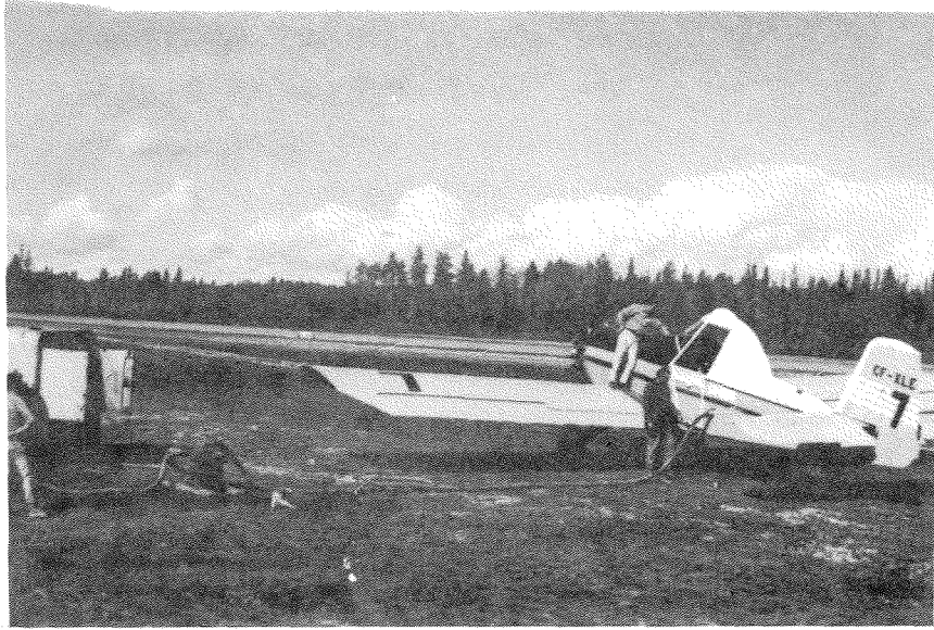
Figure 4. Thrush Commander airtanker equipped with a single drop tank.
