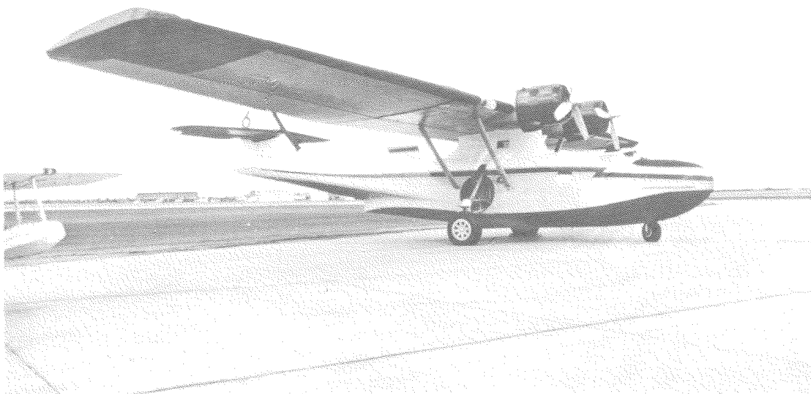
Figure 4. The twin-engine PBY5A Canso amphibian; 3637-litre (800-gal) two-compartmented tank.
