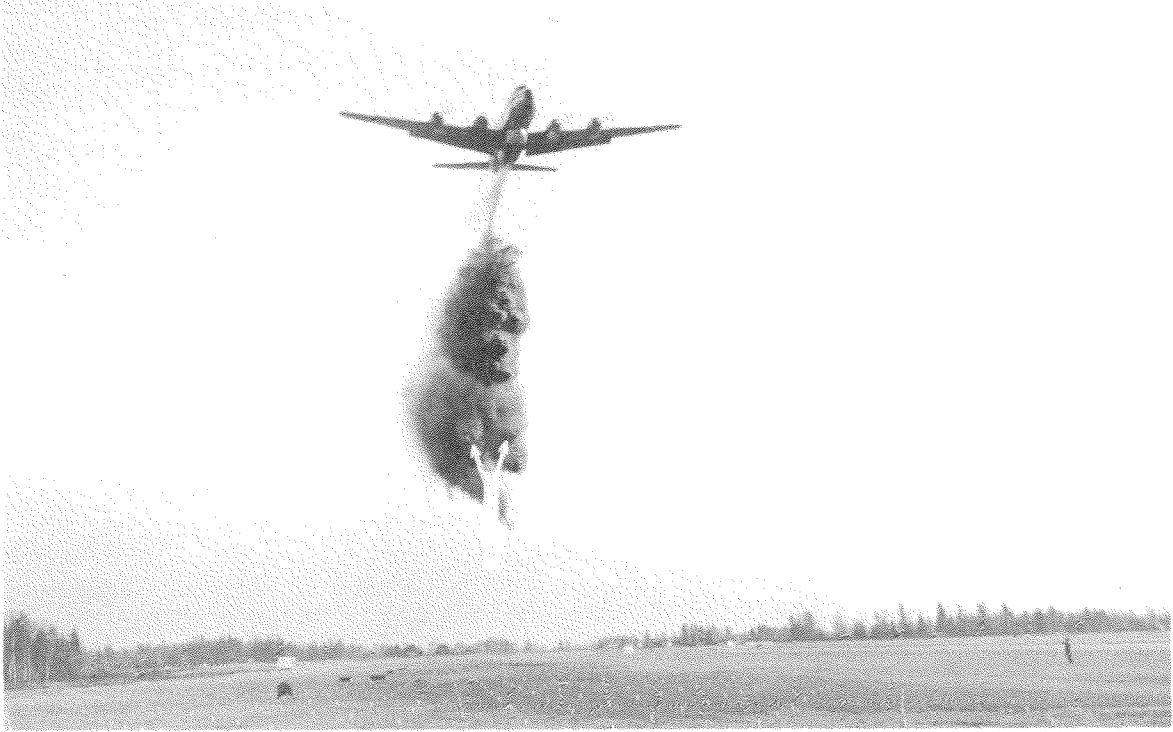
Figure 27. Individual compartments released at the same time produce a separation in the retardant mass, as in this four-door double train drop from the DC-6B.
