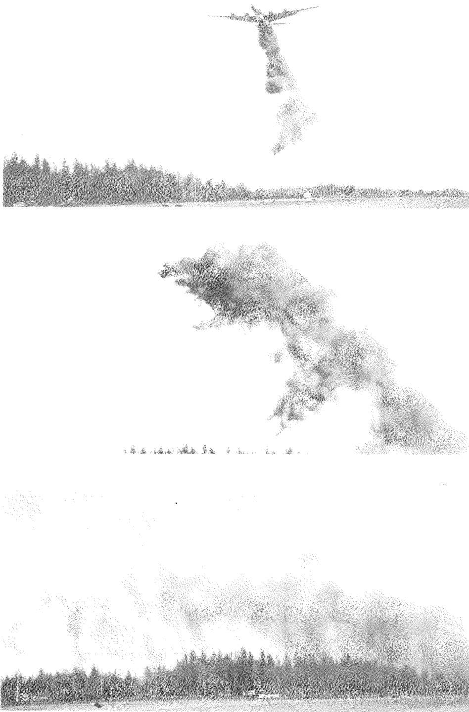
Figure 29. Four 1418-litre (312-gal) loads released in sequence from the DC-6B airtanker using manual control. Note the continuous line of retardant forming as the load reaches the ground.
