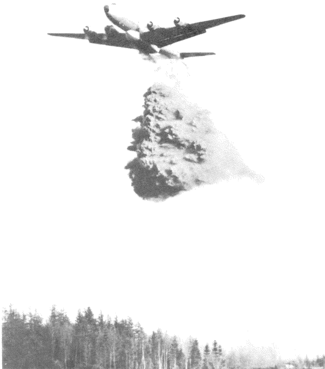
Figure 26. Sufficient venting permits large loads to be discharged "fast and clean", as with this four-door drop of 5682 litres (1250 gal) from a DC-6B.
