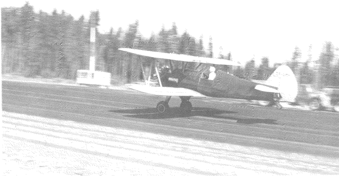
Figure 2. The single-engine Stearman; 455-litre (100-gal) single-compartmented tank.
