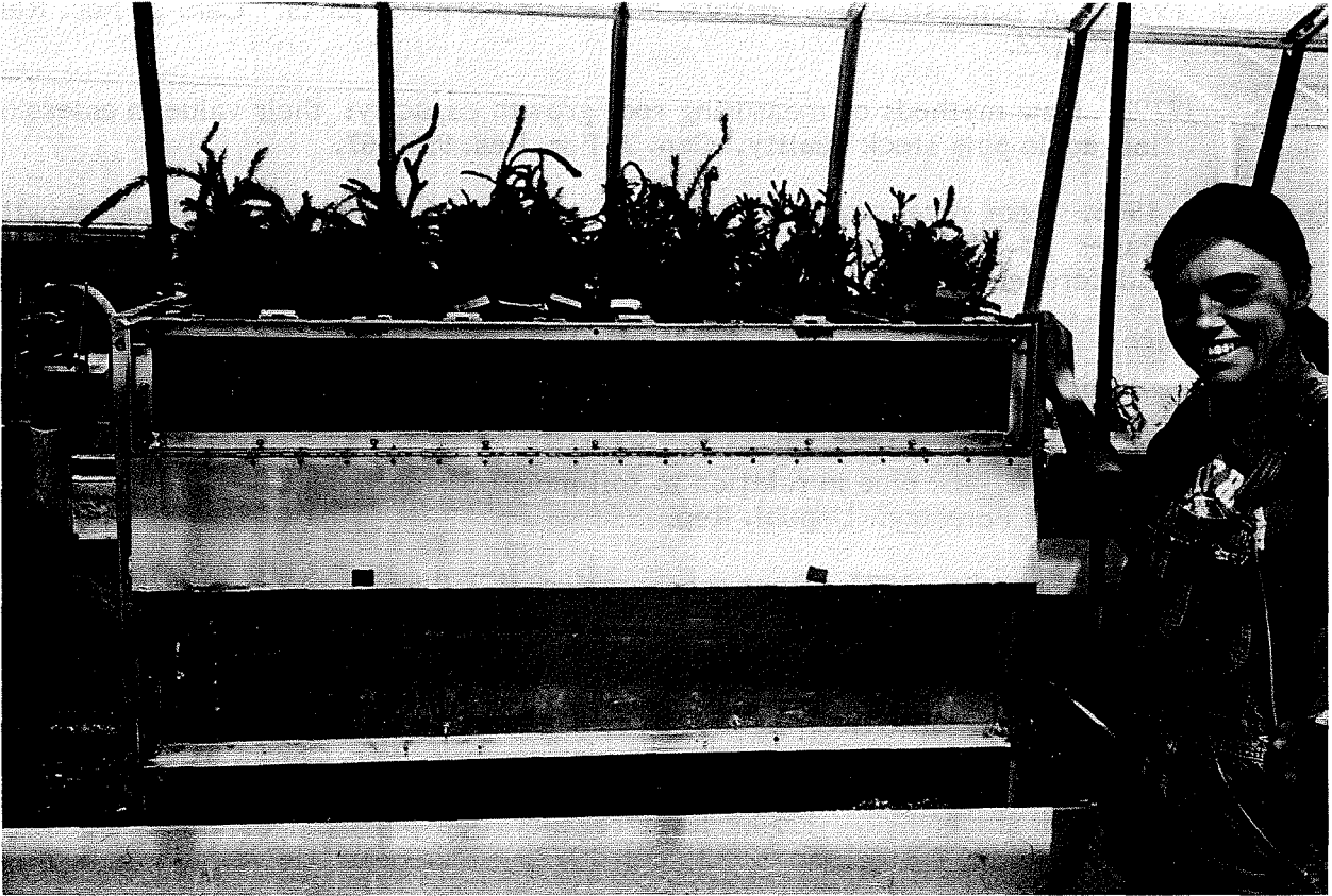
Figure 1. The root mist chamber with window exposed for viewing roots.
