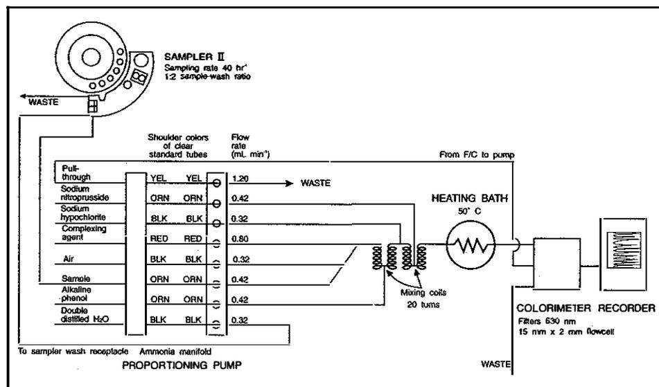
Figure 15-2. Flow diagram for the determination of NH<sub>4</sub>-N in NaCl leachates (for CEC determination) by autoanalyzer.
