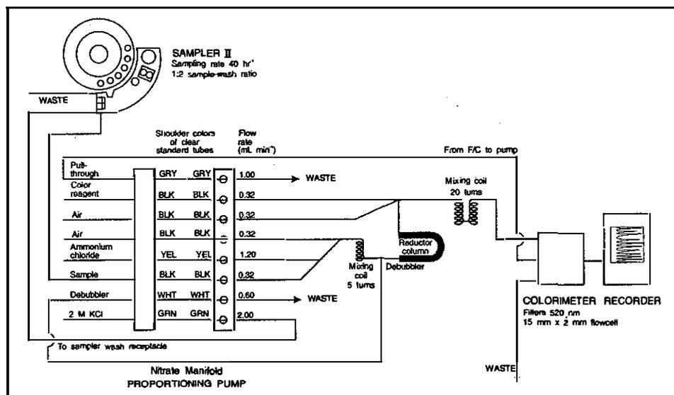
Figure 11–3. Flow diagram for the determination of NO<sub>3</sub>-N in KCl extracts by cadmium reduction.
