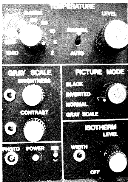
Figure 2. Controls on the display unit, which are located within easy reach of operator. No other controls need to be manipulated during flight.
