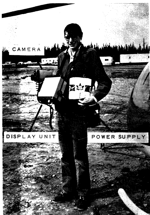
Figure 1. Components of an operational AGA Thermovision 750 system: camera, display unit, and factory-supplied power pack. Not shown is the photorecording unit. The toilet paper in the operator's hand was used for marking detected hot spots.
