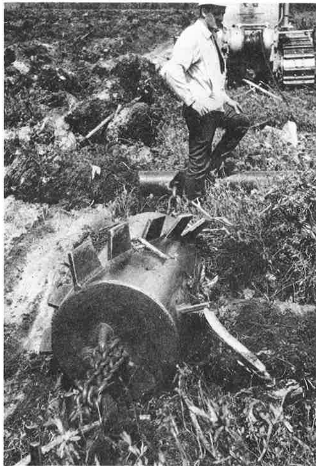
Figure 3. Shark-fin barrel and tractor pad scarifier showing combination (above) and closeup of the barrel (below).
