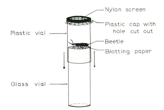
Fig. 1. A device for holding a carabid beetle in place during marking.
