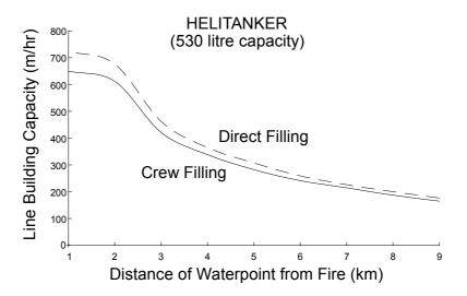
**Figure 8.** An example of the simulated productivity of a "light" helicopter with a 530-litre capacity bucket dropping water in the exotic pine plantation fuel types of southeastern Queensland (after Hunt 1986).
