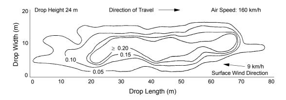
**Figure 7.** An example of a drop pattern or "footprint" for a Dromader M-18 airtanker delivering water in an open field (after Stechishen and Halicki 1984). Contour lines indicate the depth or thickness of the water concentration.
