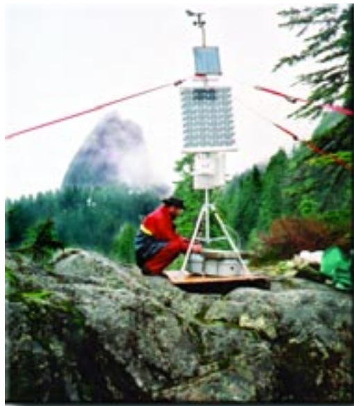
The ozone monitor and weather station being set up at 1200 metres on Alouette Mountain in Golden Ears Provincial Park.
