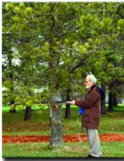
The LAI 2000 being used to measure leaf area under a pine tree.
