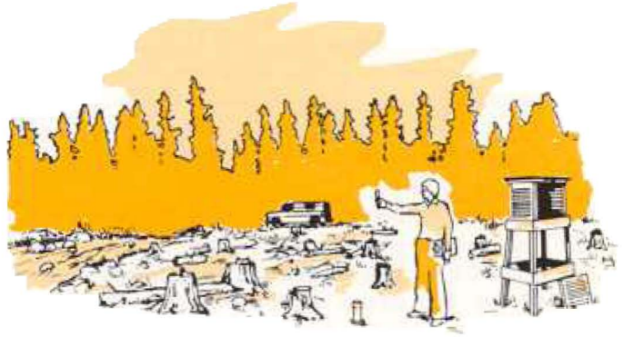
Fig. 24. Supplementary fire weather station set up in advance of prescribed burn to record weekly rainfall. Hygrothermograph in shelter. Wind measured with eye-level gauge, adding 50% to adjust to 10 m height.
