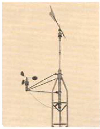
Fig. 17. Fire weather station in large clearing on open level ground. In addition to basic instruments, this station includes recording rain gauge, anemometer, solar radiation and dew recording devices. Both wire and open pole fencing were used. Vegetation has been cropped.
