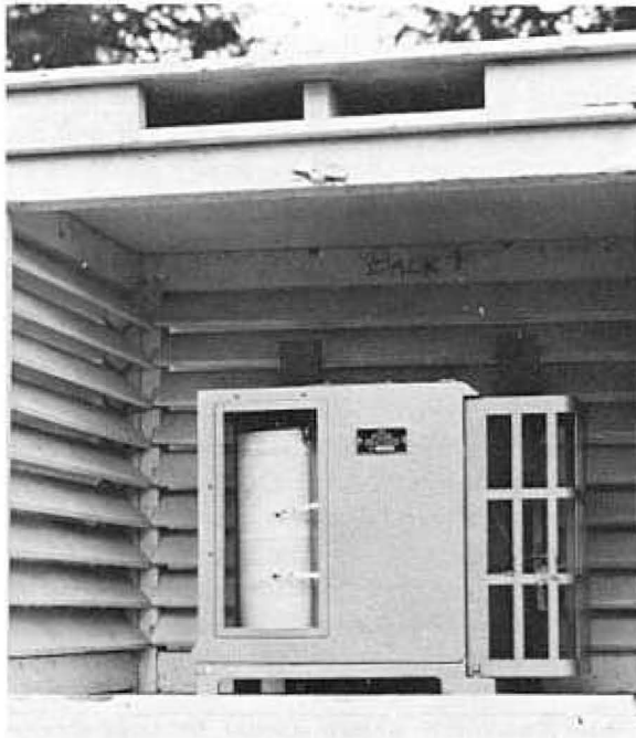
Fig. 20. Hygrothermograph mounted in separate screen. Note this is preferred type of screen with double-louvered sides and double roof.
