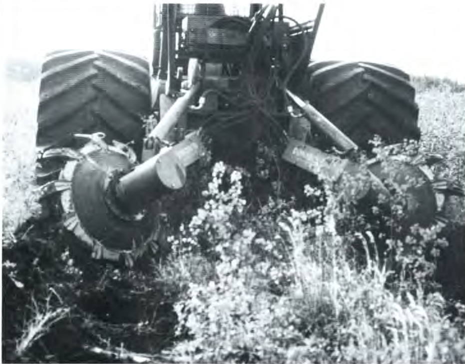
Donaren disc trencher is used for site preparation
