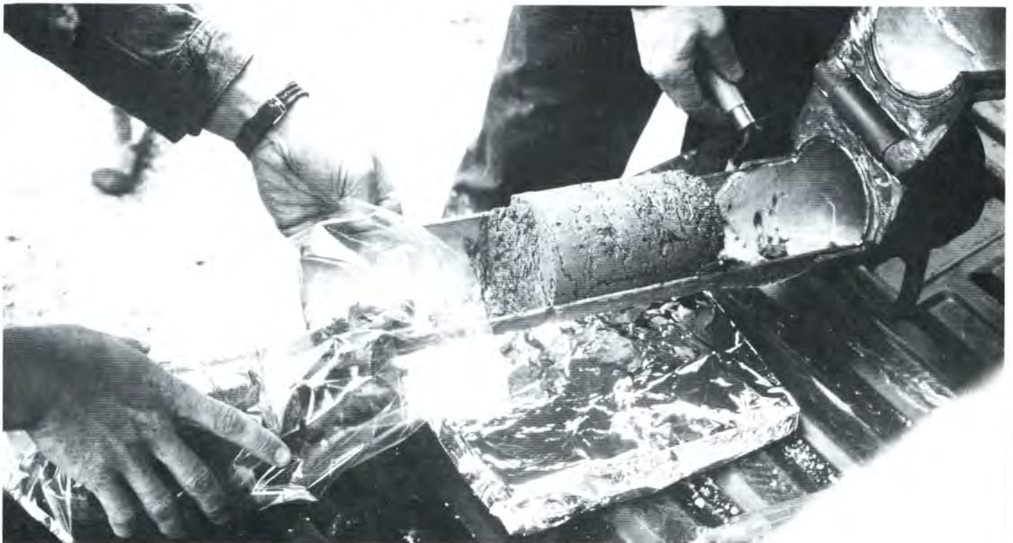
Soil core sample is taken to track movement of Pronone
