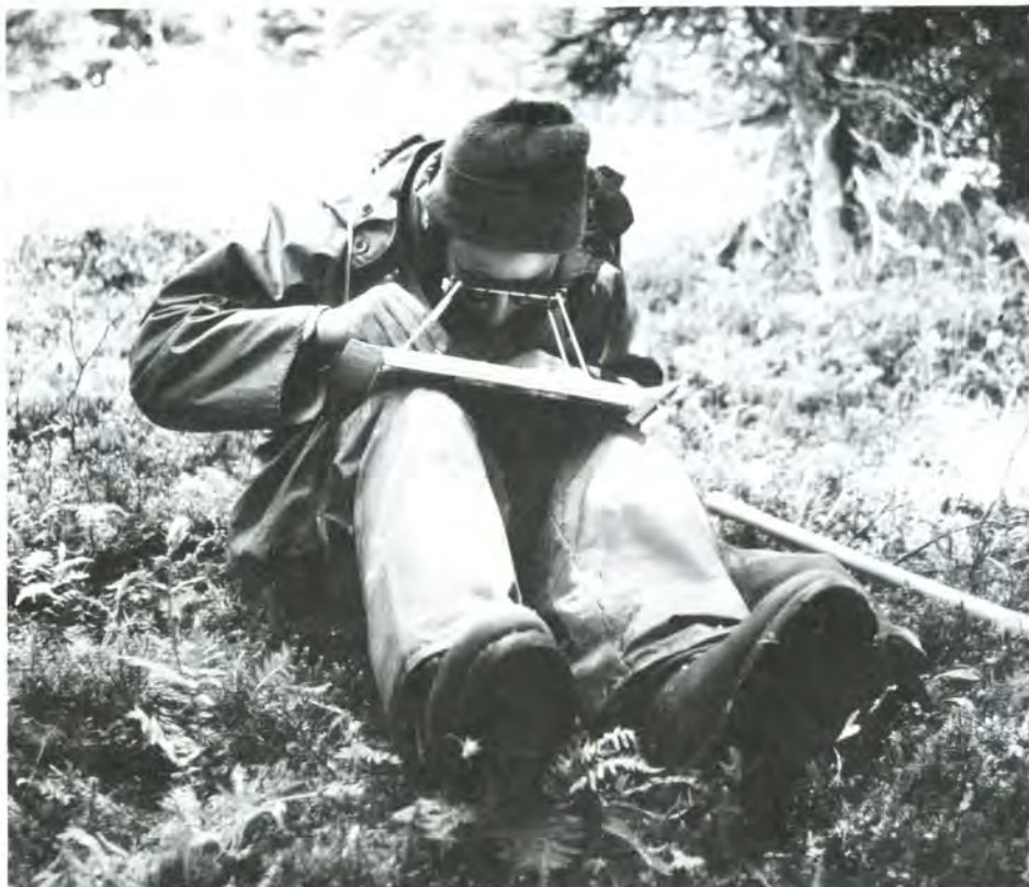
Using a stereoscope to interpret aerial photos is part of the site classification process
