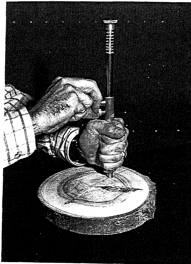
Figure 1. Wood hardness gun, or H-Gun, developed by the Northern Alberta Institute of Technology in 1990.
