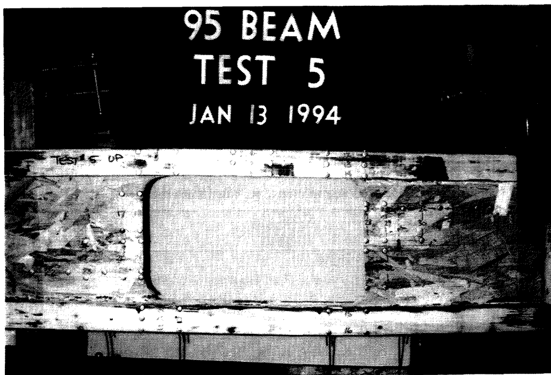
Figure 5.31. Web/flange connection failure in specimen 9.5dT5
