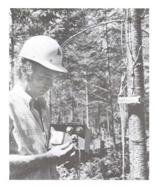
Fig. 4. Detailed measurements of weekly stem diameter growth of selected trees, using specially constructed dendrometer bands.
