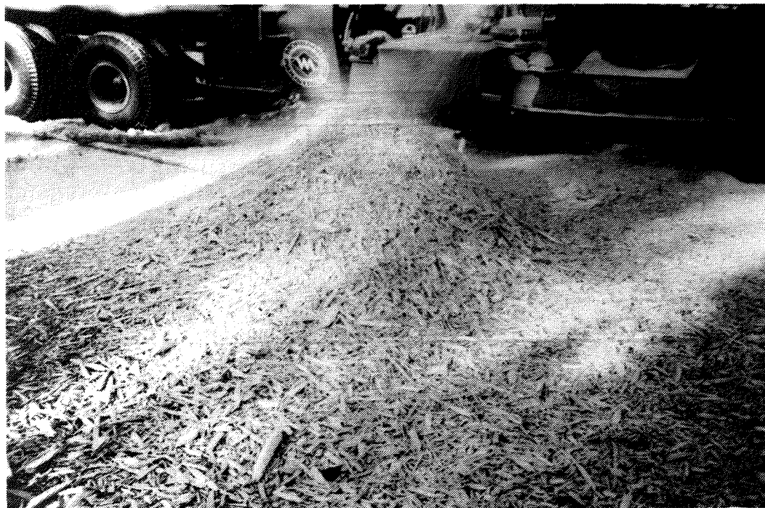
Figure 3. Chipper debris accumulating during the processing of spruce-pine full trees. Large slivers were a feature of this material.
