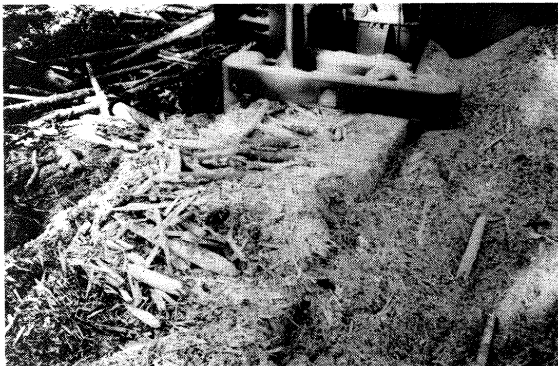
Figure 2. The extrusion of debris from the flail during the processing of spruce-pine full trees. Note the heterogeneous nature of the debris and, at the top left, the small-diameter material collecting at the feed to the flail—landing debris in the making.
