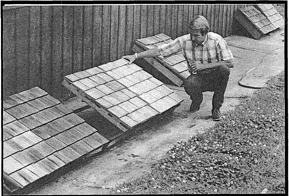
Figure 15. Pine (left), Aspen (right) Shingles on Panel for Exposure Test
