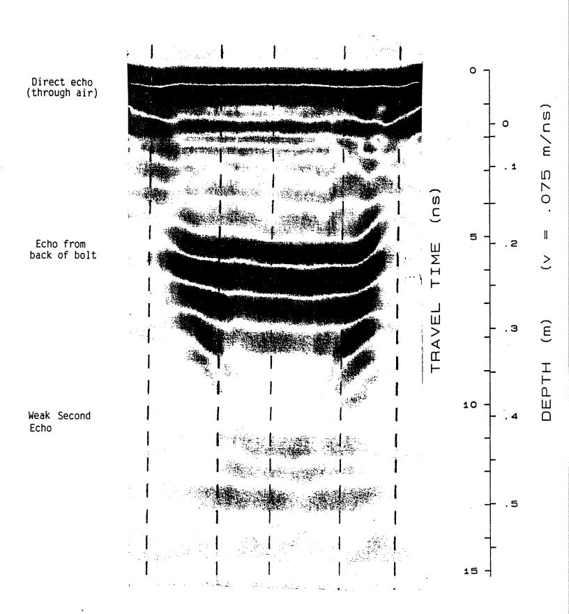
Many of the bolts studied here do not show direct and back echoes as clearly as those in Figure 2.4. In several of the records (e.g. Figures A-3, A-4, A-5) knots in the bolt appear as a distortion of the echoes. This is expected since the travel paths of the various signals are also distorted by the knot.
