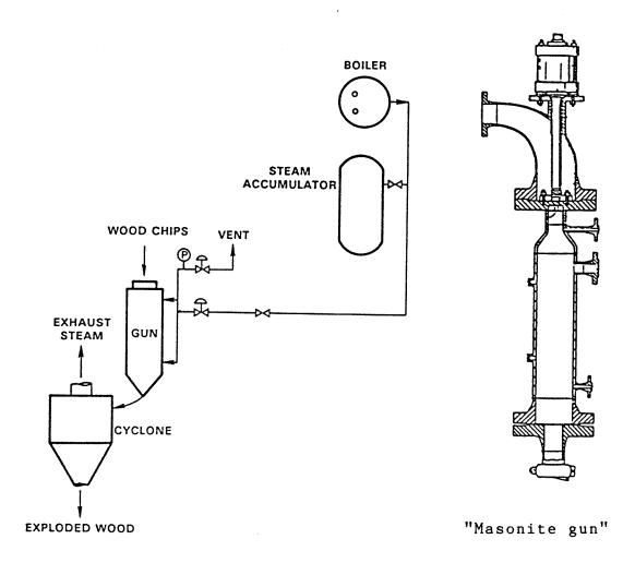
Figure 3 - Principal elements of the Tigney Pilot Plant (adapted from Ref. [8])
