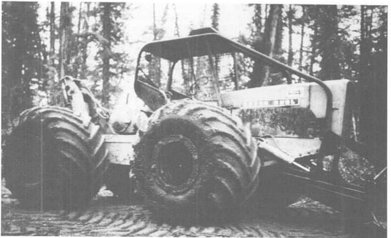
Figure 7. Goodyear HF tires were mounted on a two-piece rim with the continuous retainer outside ring.
