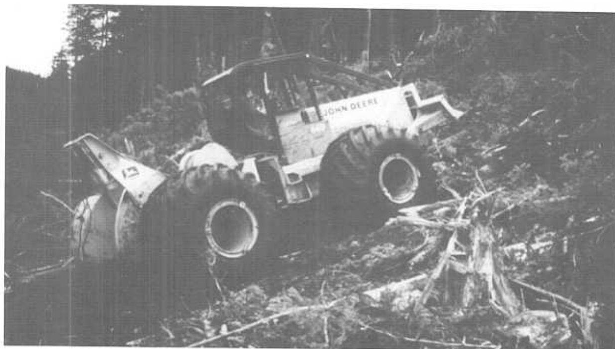
Figure 3. HF tires were installed on a JD640 skidder equipped with winch and mainline.
