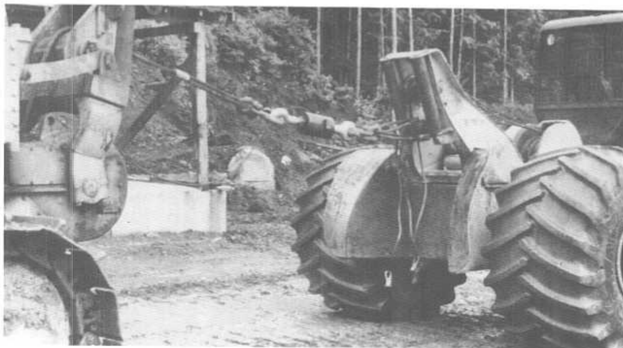
Figure 5. A load cell was used to measure and control the load applied to the skidder during traction tests.
