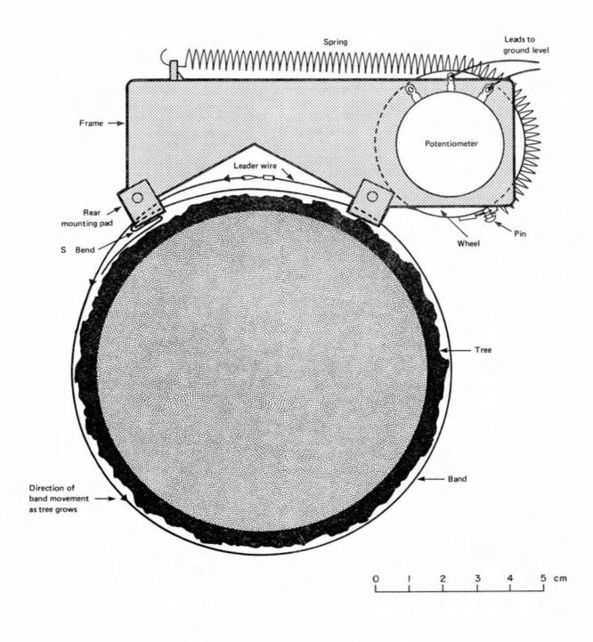
Fig. 1. The Electromechanical Dendrometer Band.
