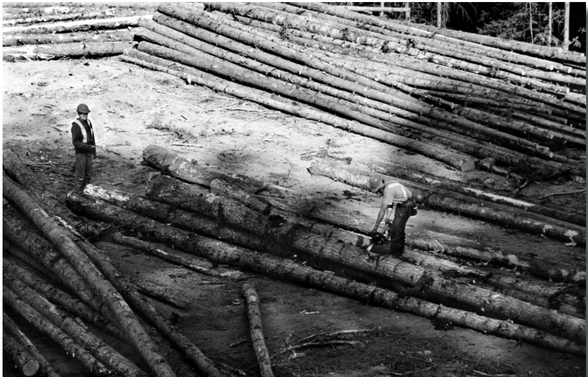
Bucking in landing.
