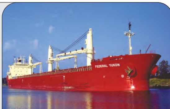
Figure 1. The Federal Yukon is typical of the newer generation of ocean-going ships of the maximum allowable dimensions to navigate the St. Lawrence Seaway. Operated by Fednav Limited of Montréal, this vessel is fitted with copper ion and sodium hypochlorite dosing systems, on an experimental basis, to test the concept of using biocides as a shipboard treatment option for ballast water of ships entering the Great Lakes. Photo by Jeff Cameron— www.wellandcanal.ca .
