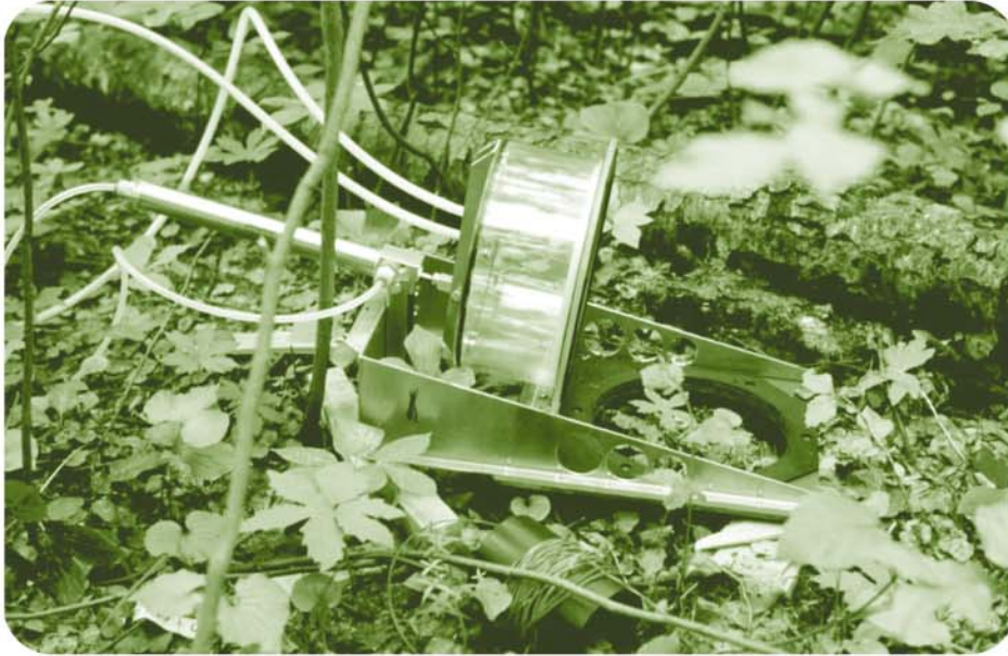
Equipment for measuring soil respiration. Photo: P.Y. Bernier
