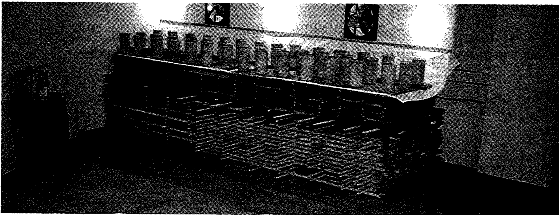
Photograph 3 - stack weighting using concrete test cylinders.
