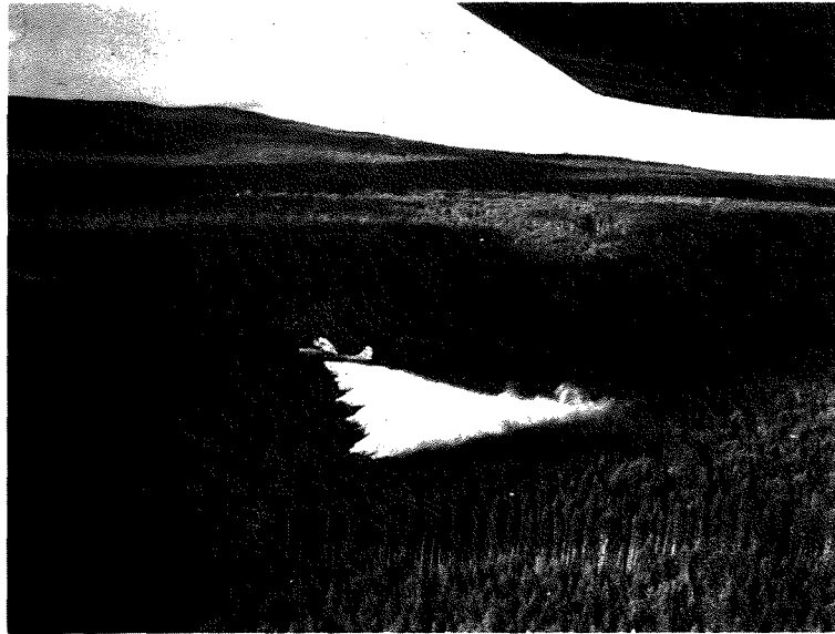
Figure 1. The 800-gal capacity PBY Canso water-bomber releasing a load of GELGARD M short-term retardant.
