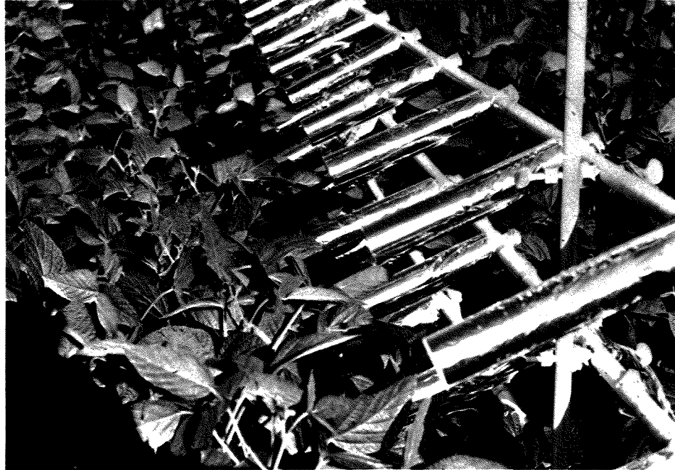
Fig. 1. Sampling system air intake manifold and radiation shields mounted in a soybean crop.
