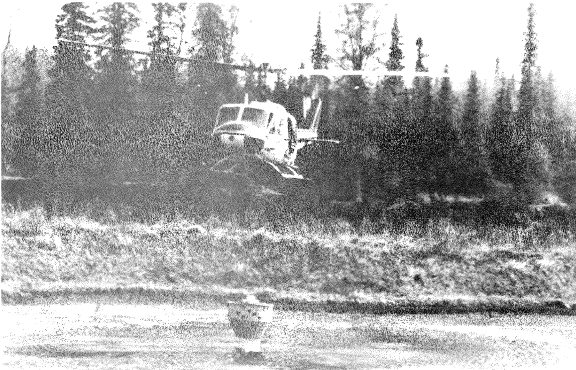
Figure 77. Bell 205A loading a bucket (Photo: Bell Helicopter Corporation).
