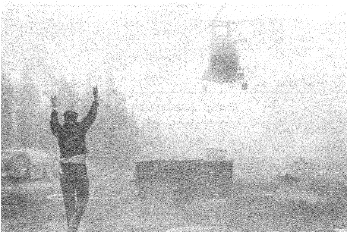
Figure 75. Kaman HH-43A twin rotor with bucket (Photo: U.S. Forest Service).
