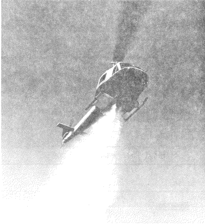
Figure 76. Bell 205A with permanently mounted tank (Photo: Bell Helicopter Corporation).
