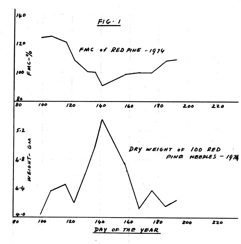
Figure 1. The trends of oven-dry weight (ODW) and foliar moisture content (FMC) for samples of 50 pairs of red pine needles taken during spring 1974.
