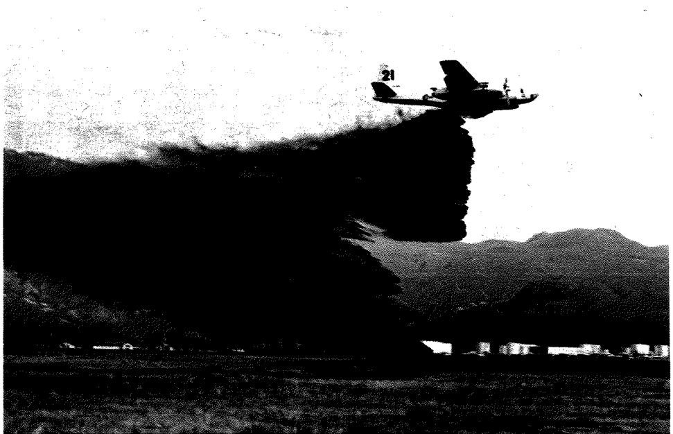
Two 450-gallon loads of Fire-Trol 100 being released in sequence (trail drop) from the B-26.
