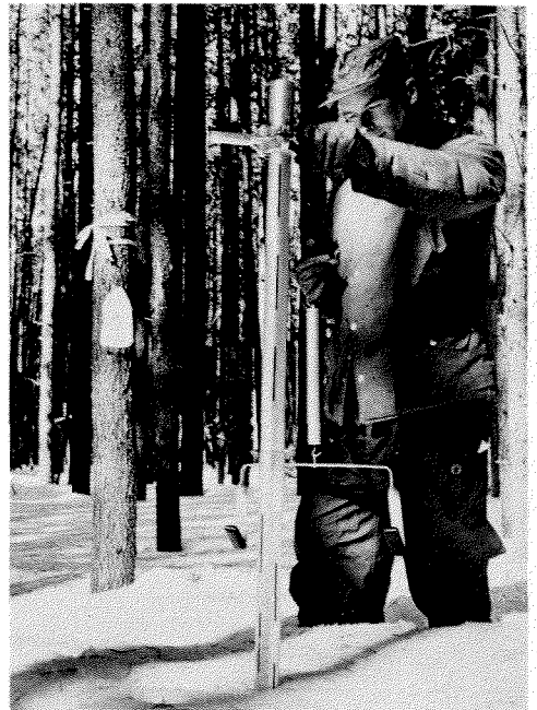
To obtain the water equivalent of the snowpack a sample is removed as a core in the snow tube and the tube with its sample is weighed with the spring balance.
