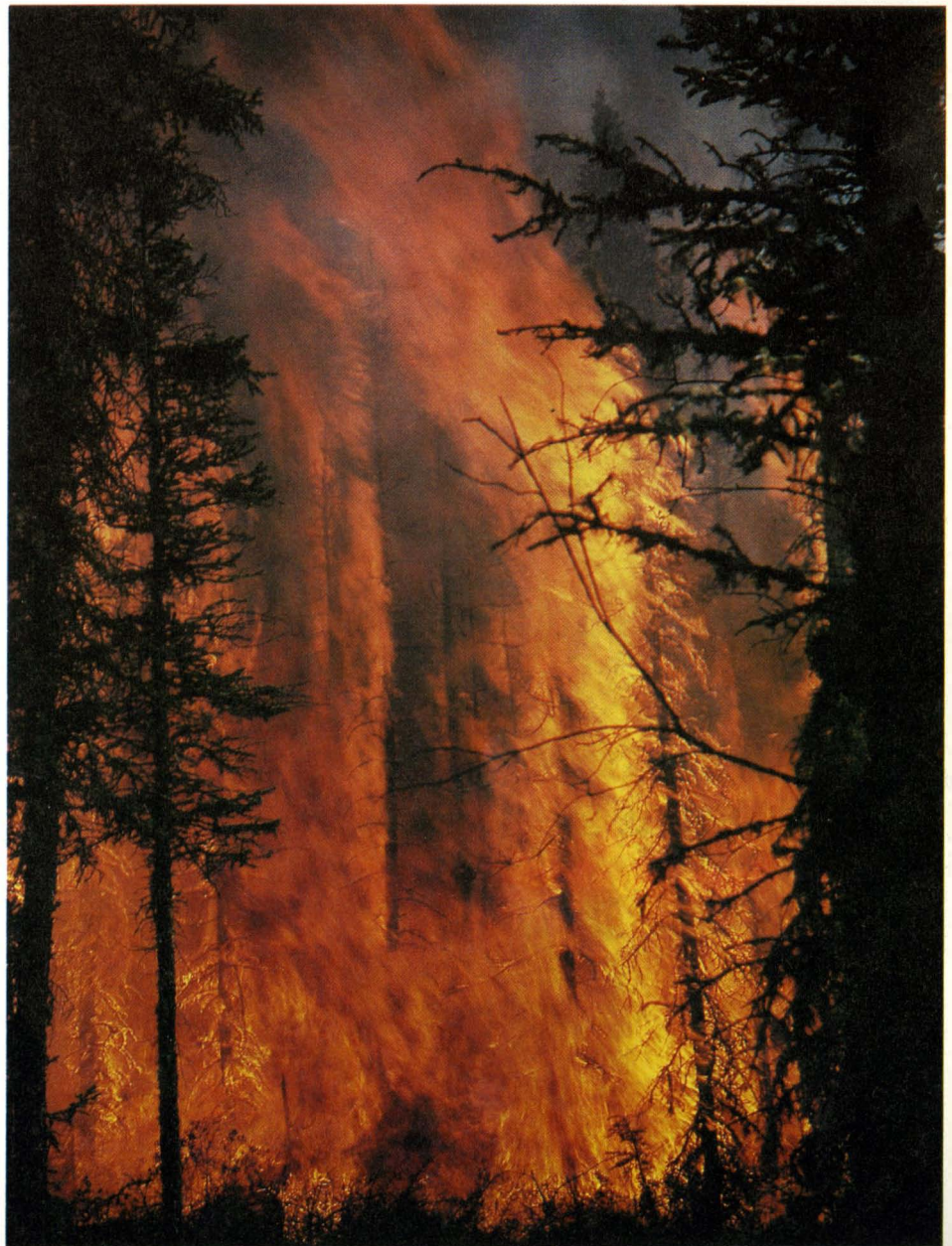
A running crown fire ignited in black spruce to test effectiveness of water and short-term retardant in inhibiting flames. In this test water and the retardant performed equally well.
