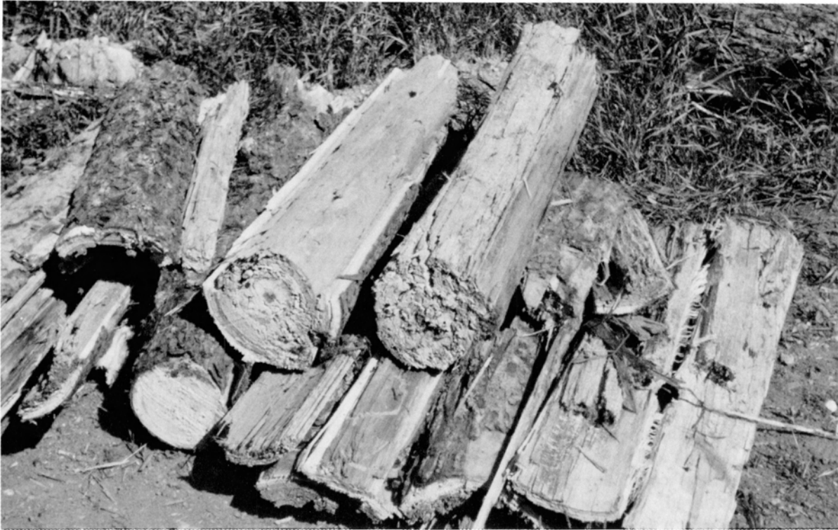
Fig. 2. Sheared Bolts of Decadent Cedar and Hemlock
