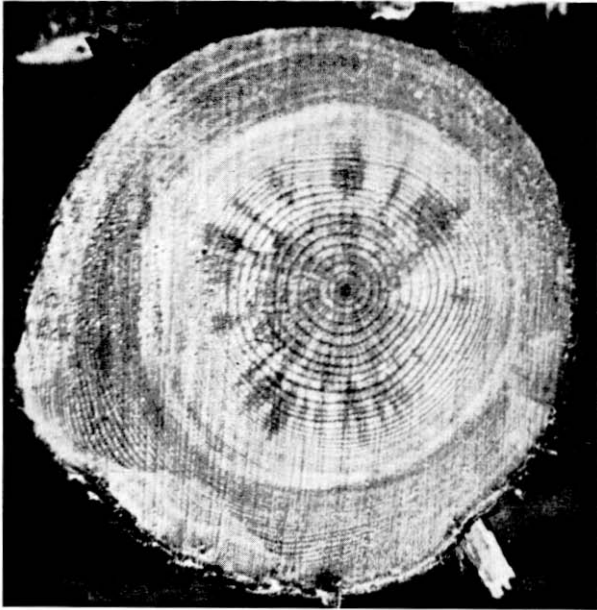
FIGURE 1. Variation in appearance of red heart stain in lodgepole pine seen upon the ends of fresh-cut logs.
