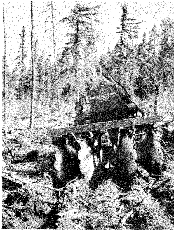
Figure 7. Tractor-drawn Athens disc plough.
