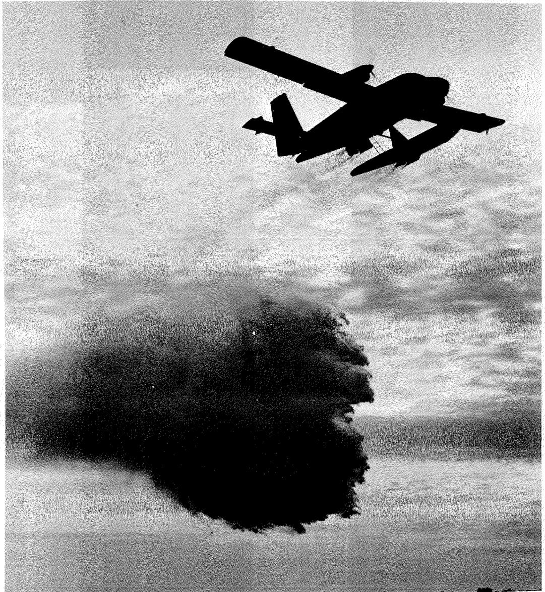
*Figure 16. 400 gallon DHC-6 Twin Otter. Note the vent flaps on the upper side of the pontoons, which open at same time as the drop doors.*
