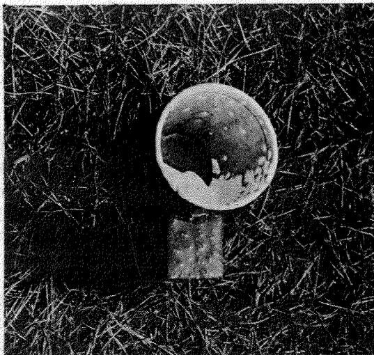
Figure 3. Collecting cup after drop from TBM Avenger with Phoschek retardant.
