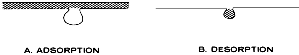
Figure 4 Diagram of a theoretical explanation for sorption hysteresis
