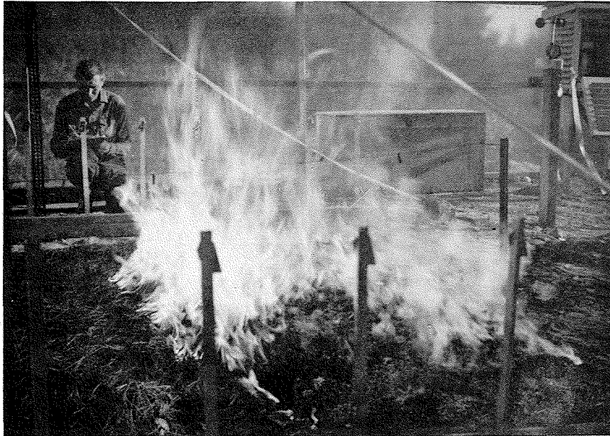
FIGURE 10 FIRE (TEST NO. 16) NOW FIVE FEET FROM IGNITION ZONE, BURNING AT 0.023 FT/SEC AT APPROXIMATE INTENSITY OF 92 BTU/FT/SEC.
