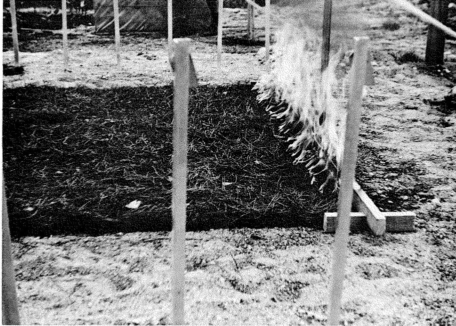
FIGURE 8 SIMULTANEOUS IGNITION OF FUEL BED AT ST. 0 (IGNITION ZONE).
