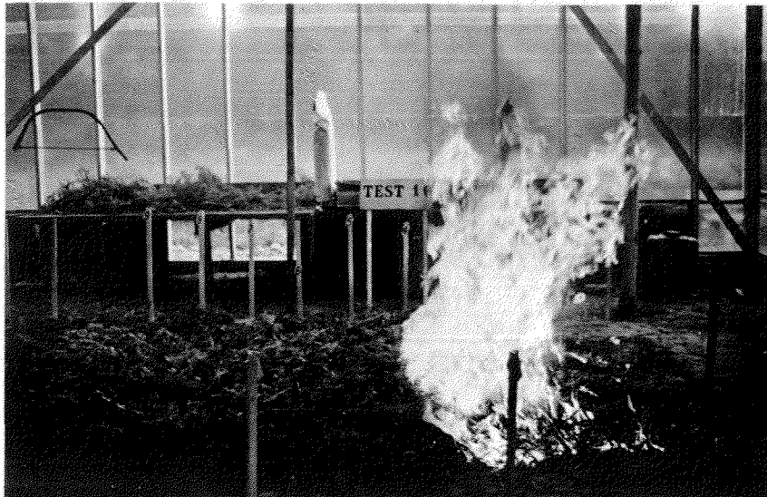
FIGURE 32. Balsam fir slash test fire burning at an intensity of 129 \text{ BTU-ft}^{-1}\text{-sec}^{-1} .
