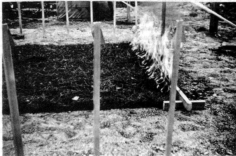
FIGURE 12. Simultaneous fuel bed ignition produced by placing a flaming, fuel oil soaked board at Station 0 (Ignition Zone).
