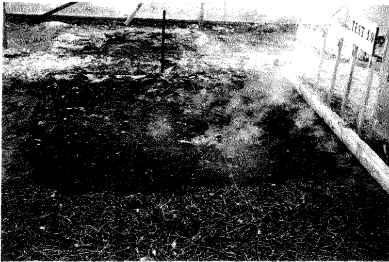
FIGURE 14. Red pine needle test fire successfully extinguished. Bed depth 2"; Applied water depth 0.027"; Temp 57°F; R.H. 88%; Intensity 53 BTU-ft -1 -sec -1 ; wind 1.6 fps; Av.ROS 0.016 ft-sec -1 ; Fuel m/c 9.4%.
