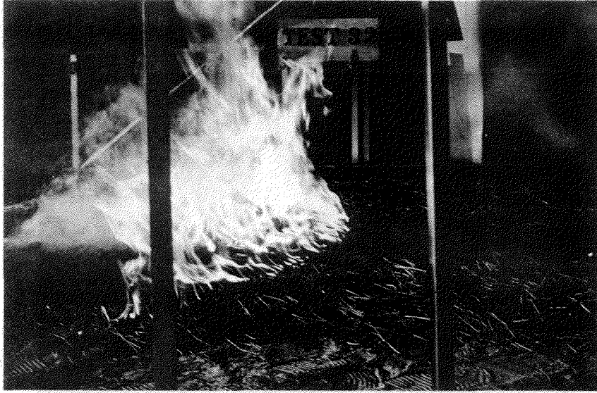
FIGURE 31. Red pine needle test fire burning at an intensity of 86 \text{ BTU-ft}^{-1}\text{-sec}^{-1} .
