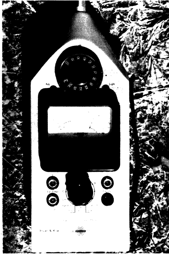
Photo No. 1. Precision sound level meter - Type 2203.
