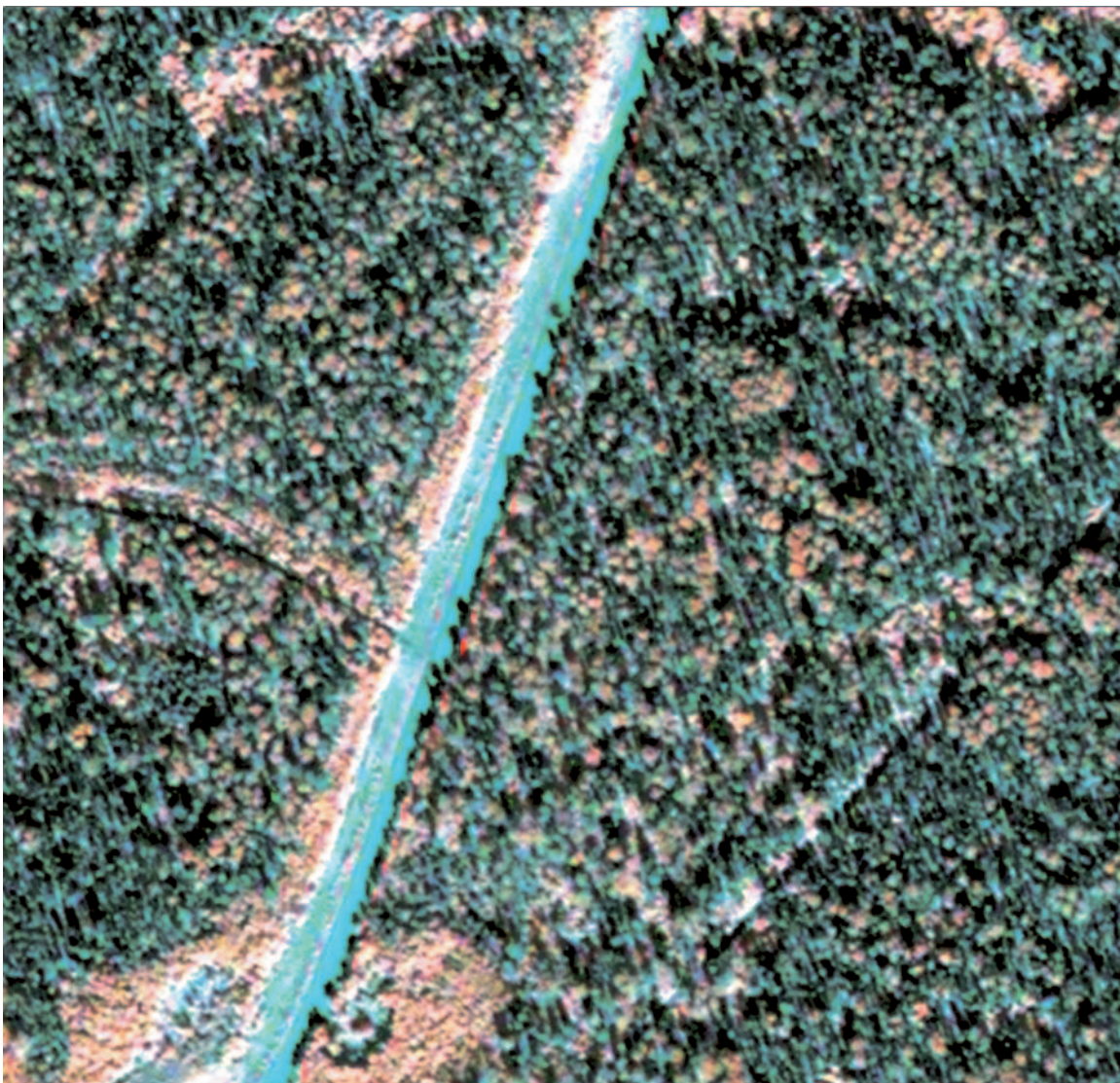
Figure 1. Subsection of the imagery showing the Brovey transformation colour infrared fused data at 0.5 m resolution (section is 410 m by 470 m).
