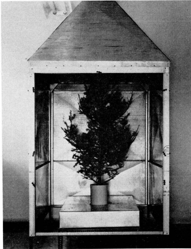
Figure 2. Laboratory flame hood with partly consumed 5-foot balsam fir.
