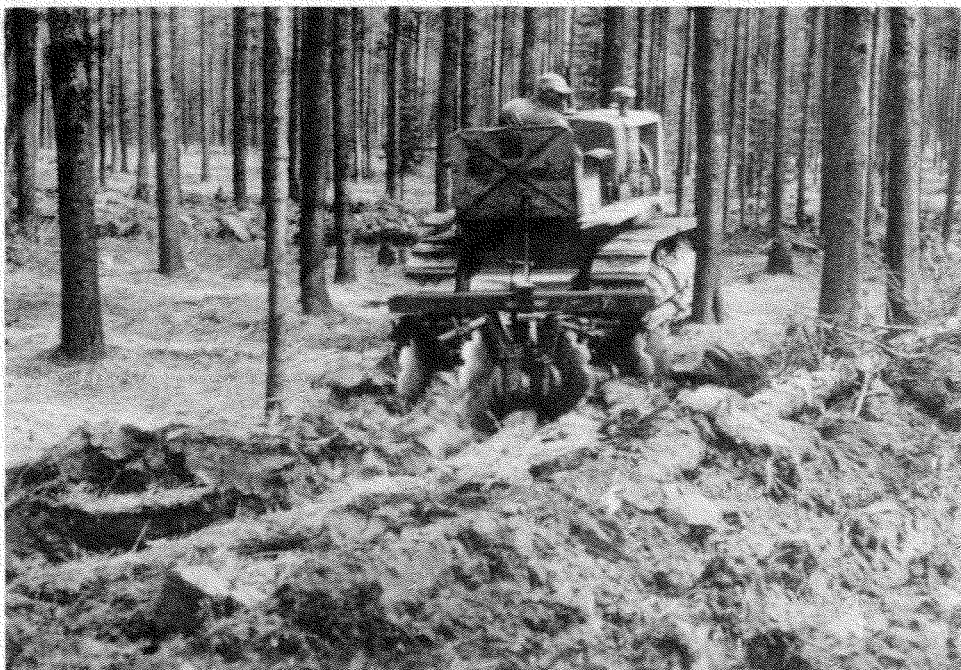
PLATE 4 – Athens type disc-plow drawn by crawler tractor scarifying the forest floor.
