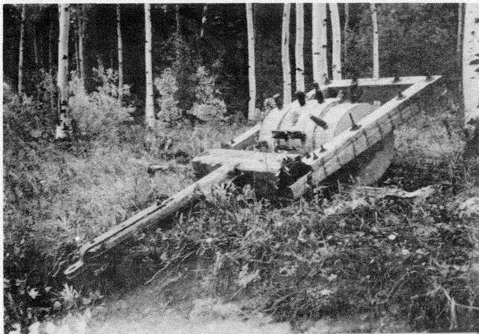
PLATE 5 – View of punch packer showing nature of punches and general construction.
