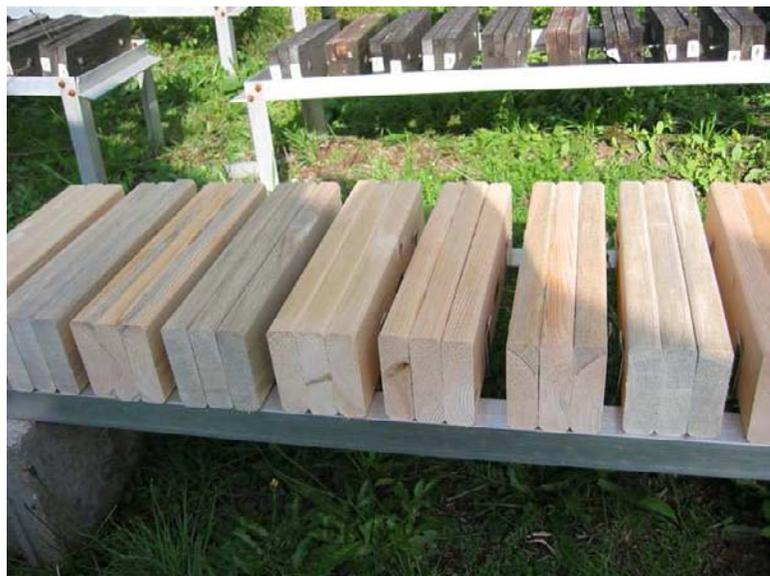
**Figure 1.** General appearance of sandwich tests in field exposure at set-up.
