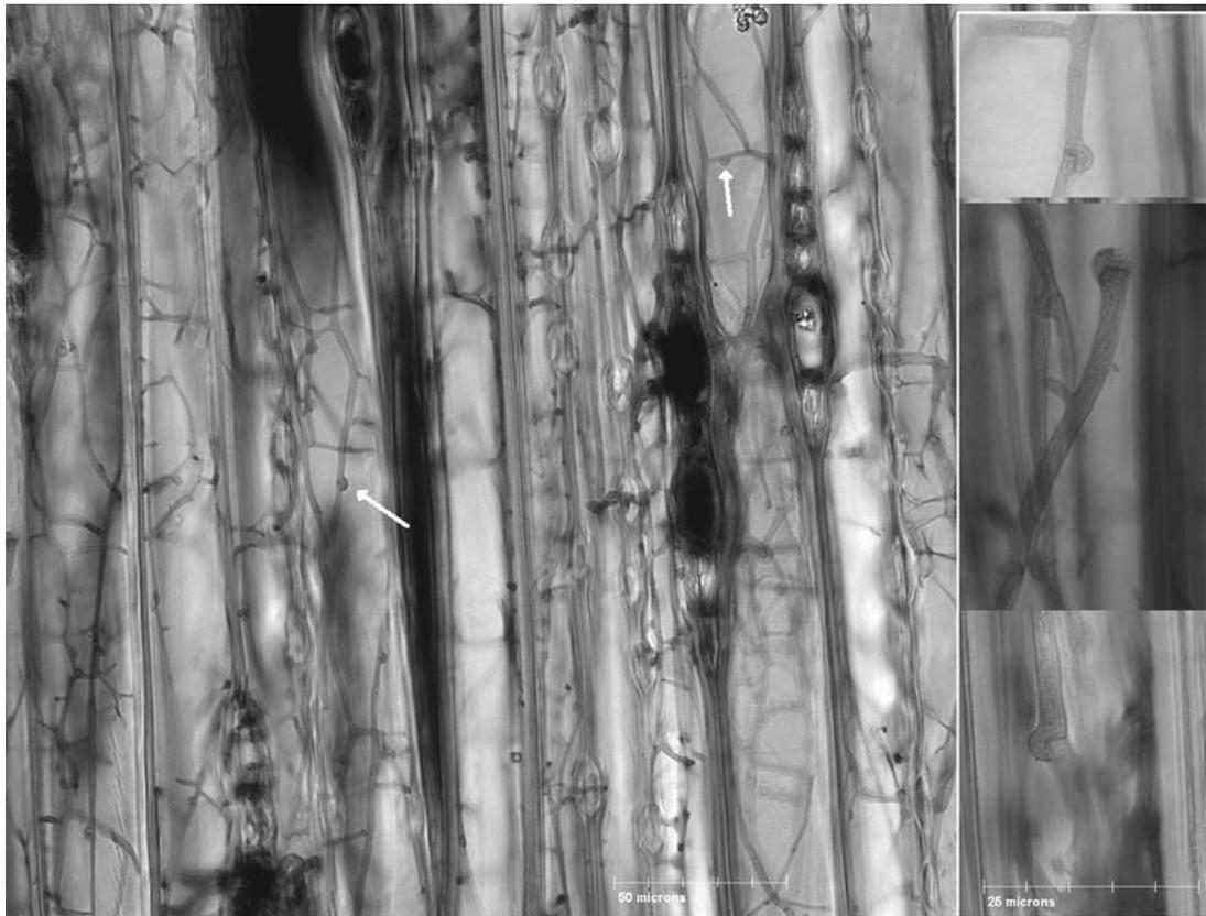
**Figure 9.** Numerous colorless hyphae (stained for observation) of brown rot fungus in cell lumina during the early stage of decay. Arrows indicate clamp connections, characteristic of basidiomycete fungi.
