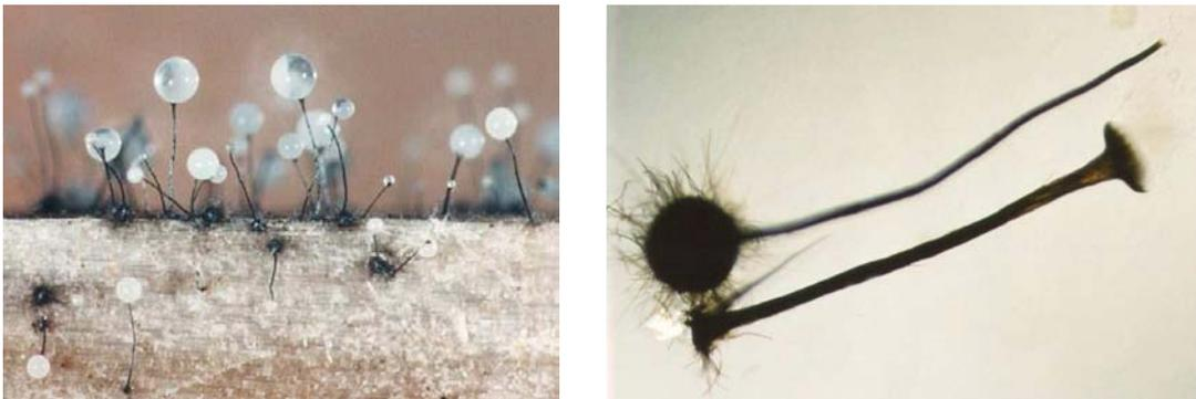
**Figure 2.** Fruiting bodies of surface bluestain fungi on green lumber. Note masses of slimy spores (left - 30x) and dark pigmentation (right - 200x).
