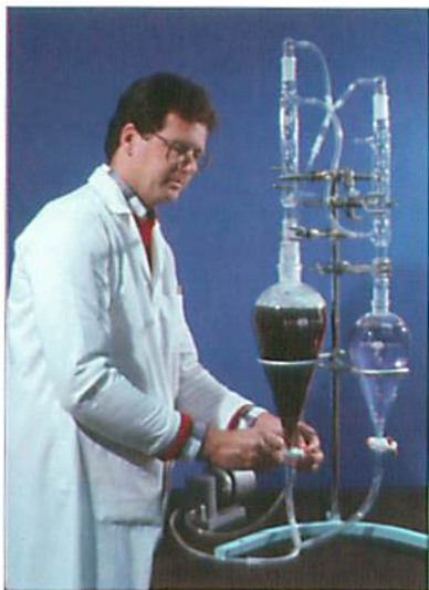
Figure 4.4 Osmotic priming is an example of seed preconditioning that produces significantly faster and more uniform germination. This technique involves the soaking of seeds in an aqueous solution of polyethylene glycol (PEG) and distilled water.
