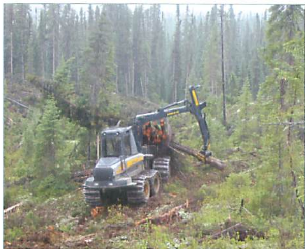
Figure 5.2 The clambunk skidder; its articulated boom eliminates damage caused by lateral sweeping and larger load capacity results in fewer passes over the site.
