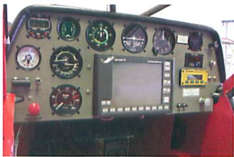
Figure 10.8 GPS-based AGNAV navigational system
