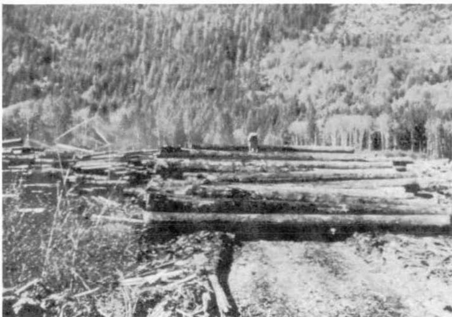
Figure 9. Log bay No. 5 partially wet (left side) from bay No. 4 spray. Comparisons were made of beetle attacks on wet and dry ends of the same logs.
