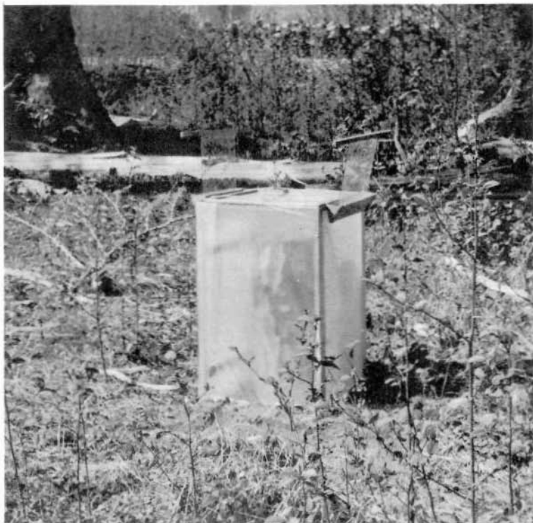
Figure 6. Indicator trap: attractive log enclosed in plastic cage with traps at screened top, for monitoring beetle flight periods.
