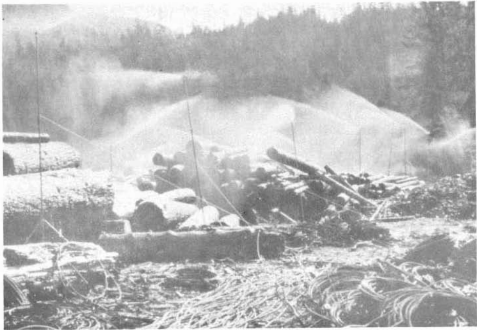
Figure 4. Log decks being sprayed, showing mist created by high pressure system.
