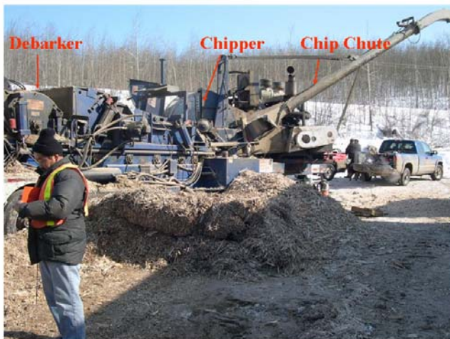
Figure 5. Petersen DDC 5000 showing debarker (A), disk chipper (B) and chip chute (C). Note the pile of hog fuel in the center of the picture.
