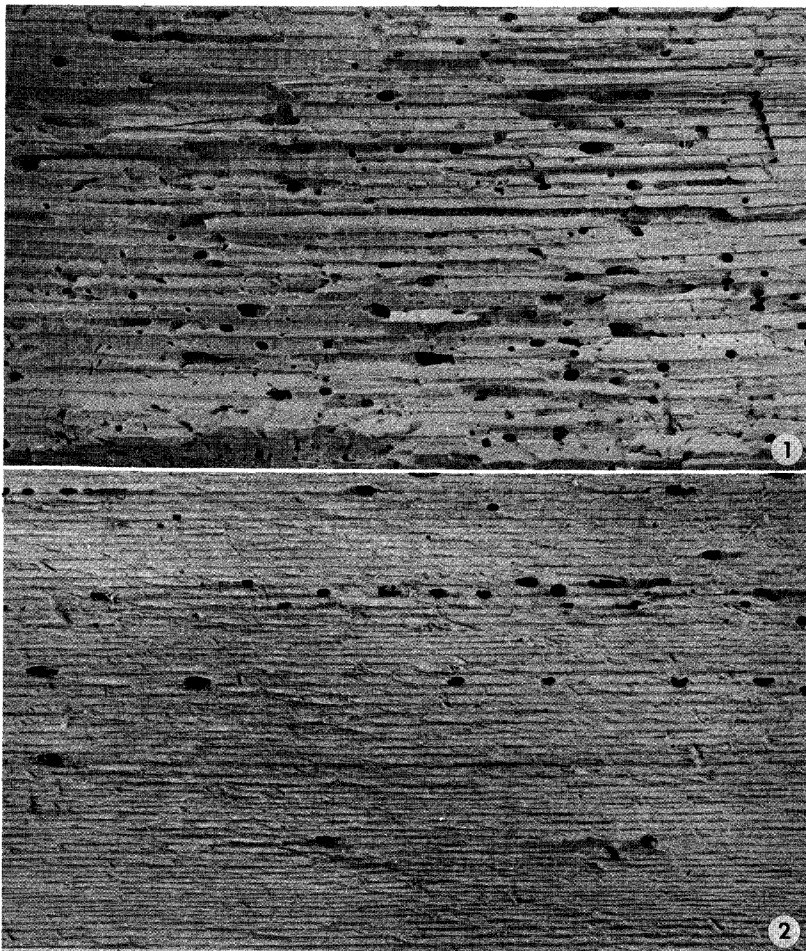
Figure 1. Damage caused by a weevil, Hexarthrum sp., in log of old growth western red cedar, Revelstoke, Central Nelson District, July 1959. J. C. Holms.
