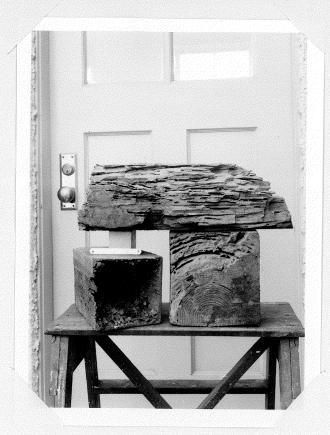
Showing sample sections of termite damaged foundations timbers removed from buildings in Vancouver, B.C.
